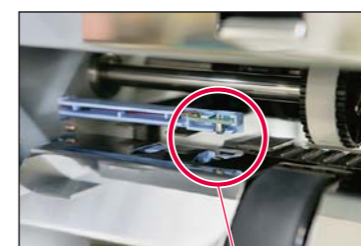
Double Feed Detect Sensor
